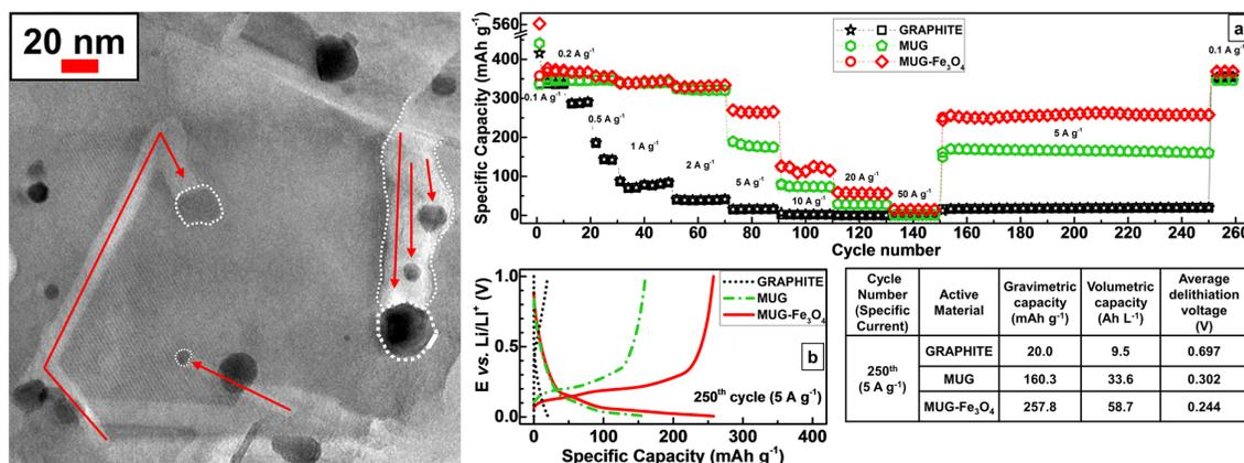
Figure 1: MUG-Fe<sub>3</sub>O<sub>4</sub> TEM micrograph. Fe<sub>3</sub>O<sub>4</sub> nanoparticles are outlined with white round dot dashes and, the carving paths, are indicated with red arrows
