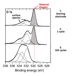
XPS O 1s spectra of LMR-NMC electrodes before cycling, and after 1 cycle and 165 cycles, in half cells with EC/PC/EMC/DMC + 1M LiPF<sub>6</sub> + 5 wt. % TTFP electrolyte
